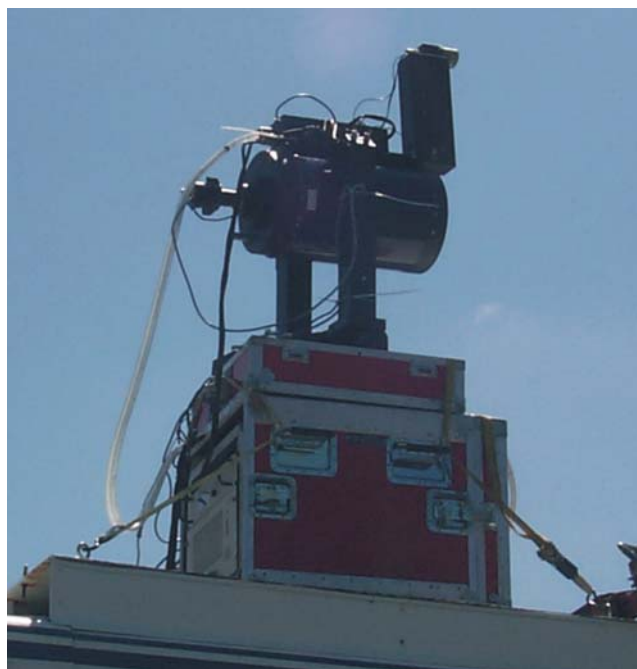
Figure 2. A photograph of the miniature elastic lidar set up to map particulates in the field. This instrument took the data in figures 1 and 2.
