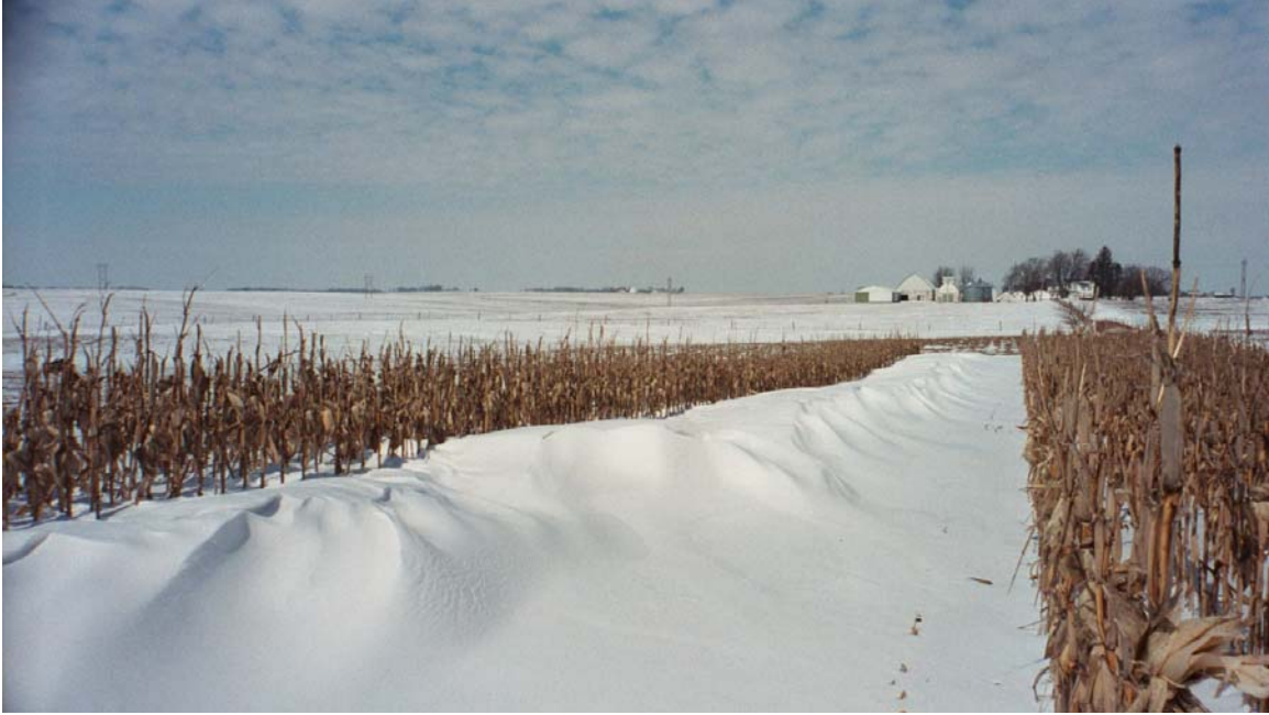
Figure 3.6: Year 1 Tests, two sets of eight rows of corn with an 8 row gap between
