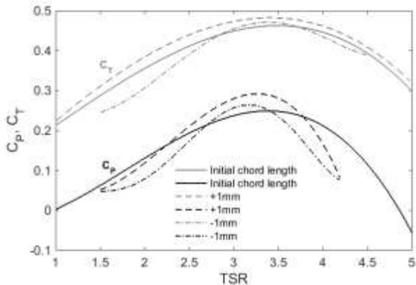
Figure 7. Sensitivity of  $C_p$  and  $C_T$  to changes of chord length for  $\pm 1$  mm (Commercial turbine);
