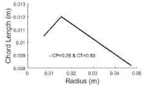
Figure 4. Chord length distribution of the designed turbine model
