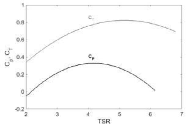
Figure 6. Variation of power and thrust Coefficient versus tip speed ratio for the designed turbine's model
