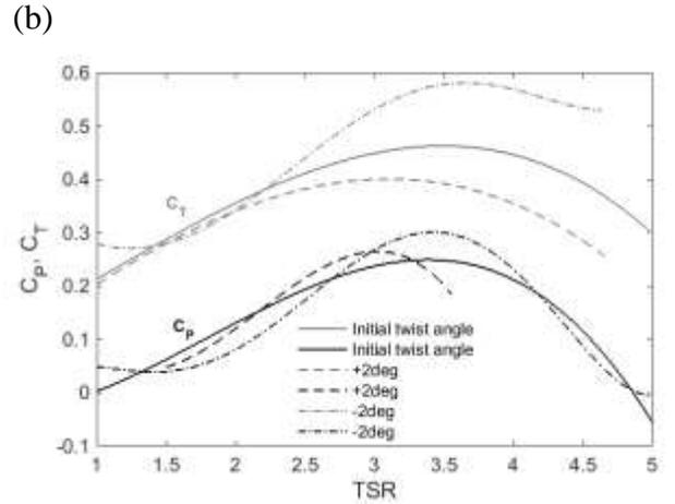
Figure 8. Sensitivity of  $C_p$  and  $C_T$  to the changes of twist angle for  $\pm 2^\circ$  (commercial turbine)
