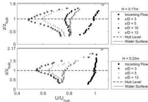
Figure 9. Mean streamwise velocity profiles in the wake of a commercial model turbine for 0.17 m and 0.23 m flow depths.
