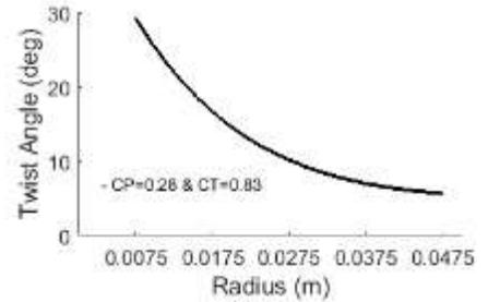
Figure 5. Twist angle distribution of the designed turbine model
