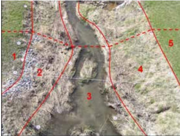
Dispose bench marks, also called Ground Reference Points (GRP), on the field. Each of the plans should be defined by at least 6 spatially well-distributed GRPs to allow an accurate orthorectification (see Fujita, 1994). Take a picture of the site and store this picture in the folder *Map*.
