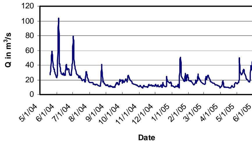
Figure 8. The typical annual cycle in the Alec River (June 1<sup>st</sup>, 2004 – May 31<sup>st</sup>, 2005), the mean daily inflow within the year was  $18.9 \text{ m}^3/\text{s}$ .
