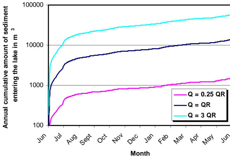
Figure 19. Annual cumulative amount of sediment enters (trap) into the lake under different flow conditions,  $Q_R = 18.9$   $m^3/s$ .
