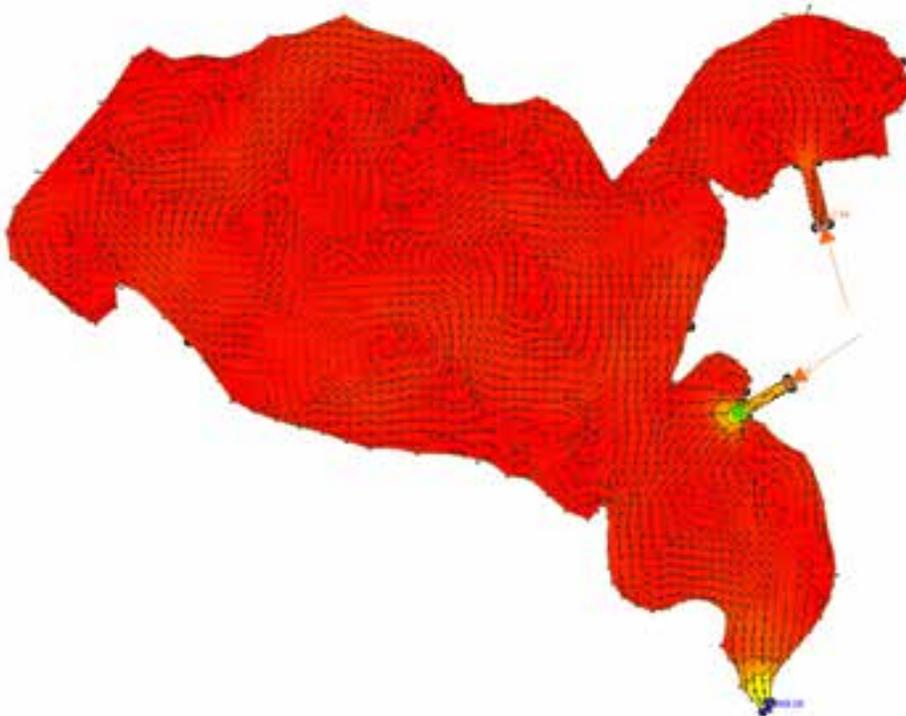
Figure 30. Re-circulation pattern for event -3;  $Q_T = 6.74 \text{ m}^3/\text{s}$ .
