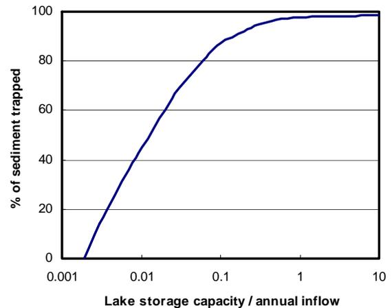
Figure 12. Trap efficiency of reservoirs as a function of the ratio of annual inflow to reservoir storage capacity.
