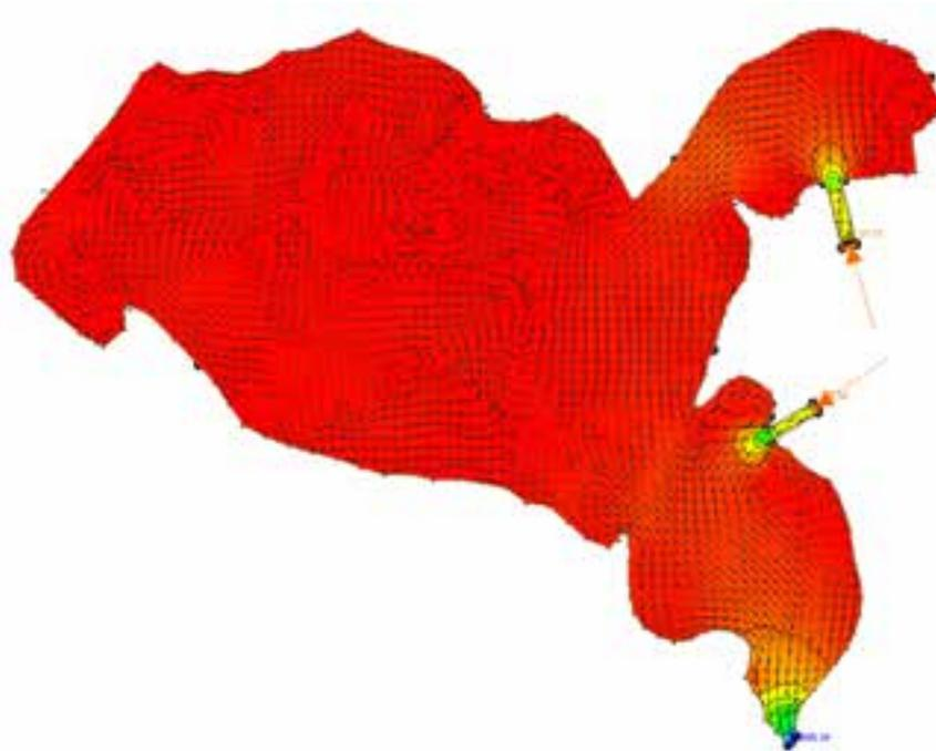
Figure 28. Re-circulation pattern for event -1 ;  $Q_T = 68.16 \text{ m}^3/\text{s}$ .
