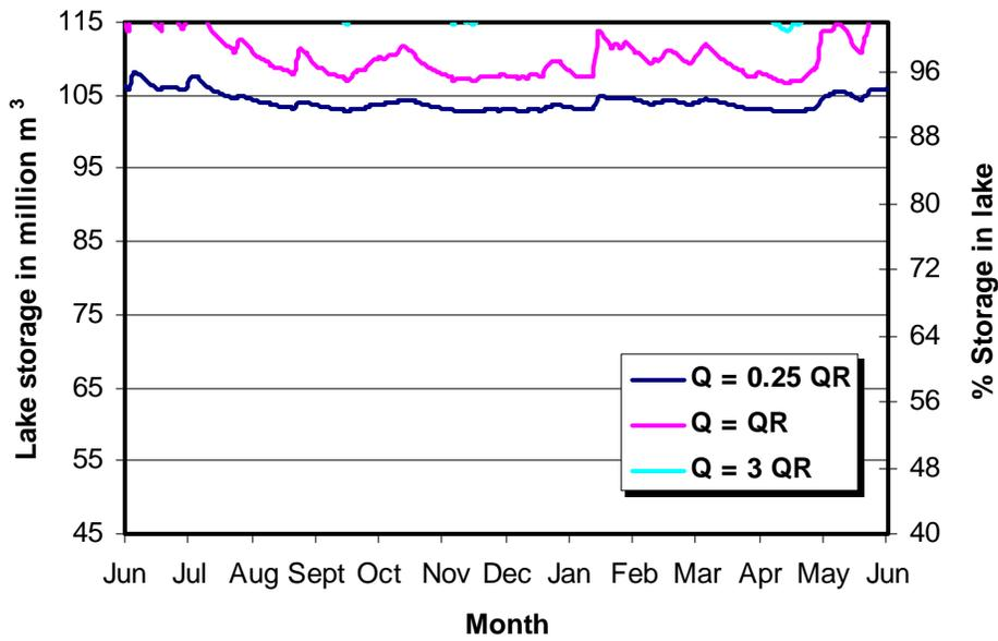
Figure 18. Black Lake water storage for the exit base-level ( $E_{le} = 1000$  m;  $S = 100$  millions  $m^3$ ) under different flow events,  $Q_R = 18.9$   $m^3/s$ .
