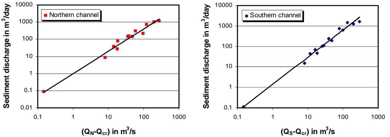
Figure 15. Sediment discharge- inflow discharge relationships for Alec northern and southern channels.
