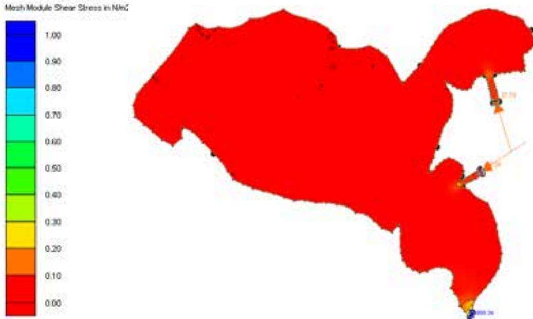
Figure 25. Shear stress distribution in the lake and its inlets and exit;  $Q_T = 68.16 \text{ m}^3/\text{s}$ ; dimensions in  $\text{N}/\text{m}^2$ .
