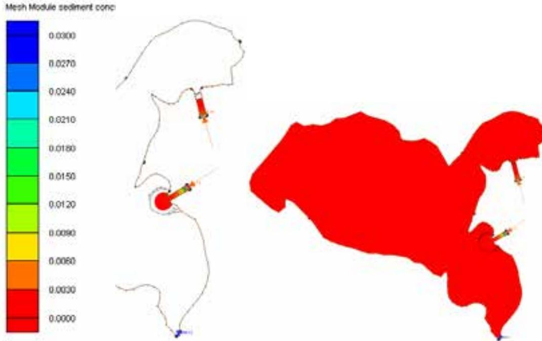
Figure27. Sediment concentration distribution in the lake and its inlets and exit (event -2);  $Q_T = 20.42 \text{ m}^3/\text{s}$ ; dimensions in  $\text{ppm} \times 10^3$ .
