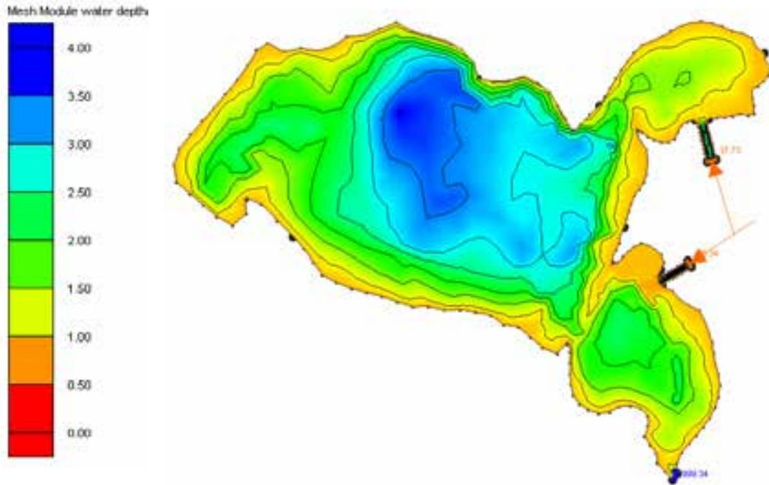
Figure 21. Water depth in the lake (event-1);  $Q_T = 68.16 \text{ m}^3/\text{s}$ ; dimensions in m.
