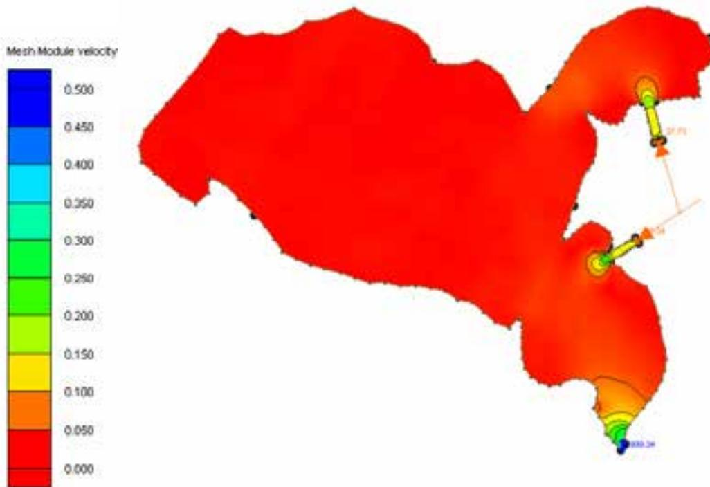
Figure 22. Velocity distribution in the lake and its inlets and exit (event-1);  $Q_T = 68.16 \text{ m}^3/\text{s}$ ; dimensions in m/s.
