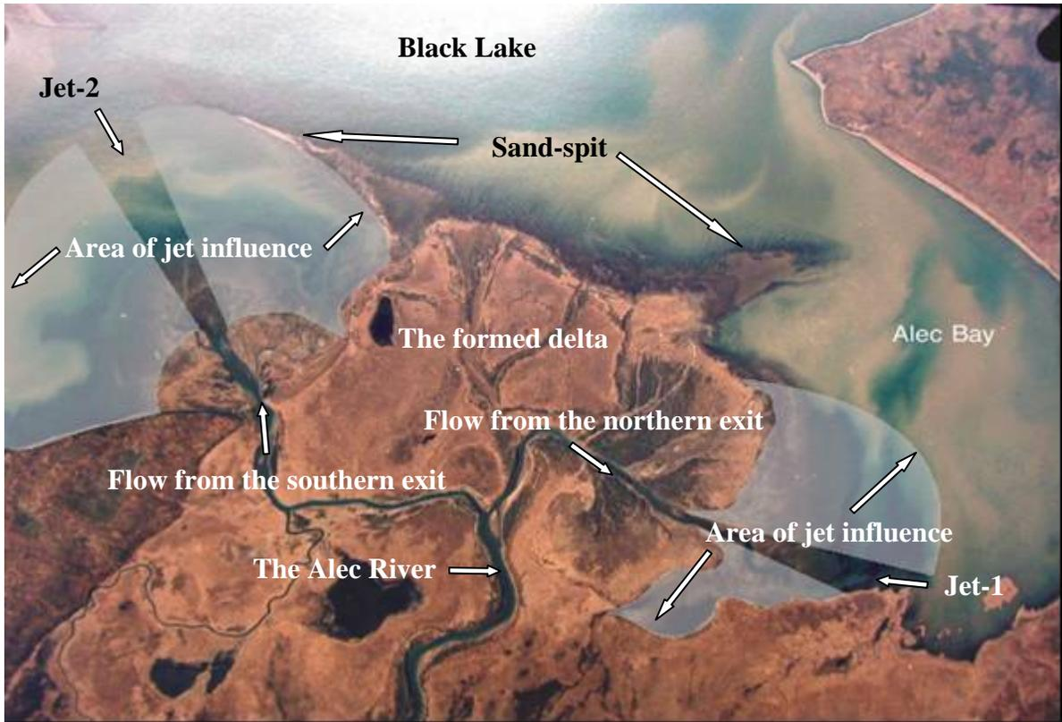
Figure 13: Aerial photo for the Alec River exit into the Black Lake showing the formed delta, sand-spit, water jets and their extended influence inside the lake.
