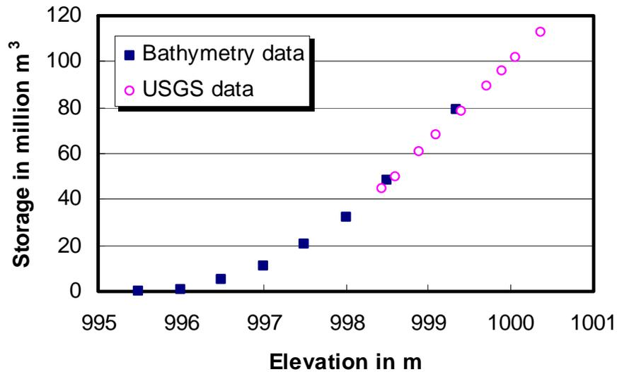
Figure10. Elevation-storage relationship.
