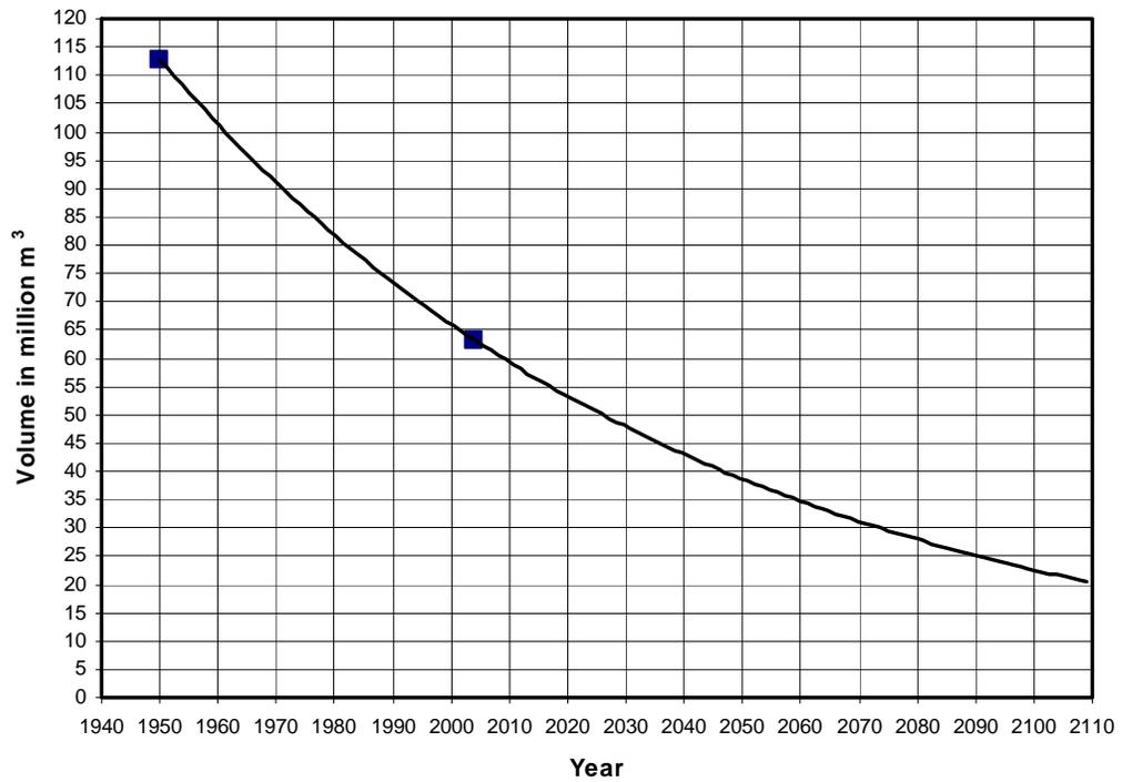
Figure 31. Expected possible change in the Black Lake water volume with respect to time (exponential fit).
