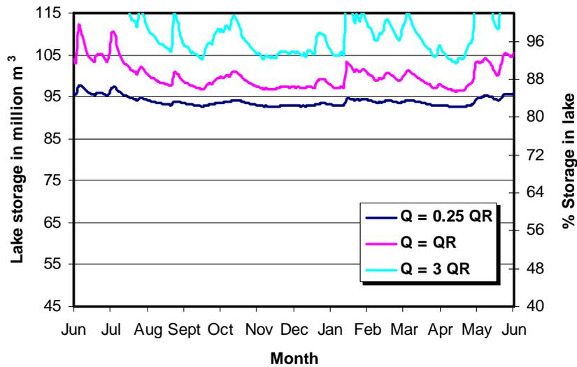
Figure 17. Black Lake water storage for the exit base-level ( $E_{le} = 999.75\text{m}$ ;  $S = 90$  millions  $\text{m}^3$ ) under different flow events,  $Q_R = 18.9 \text{ m}^3/\text{s}$ .
