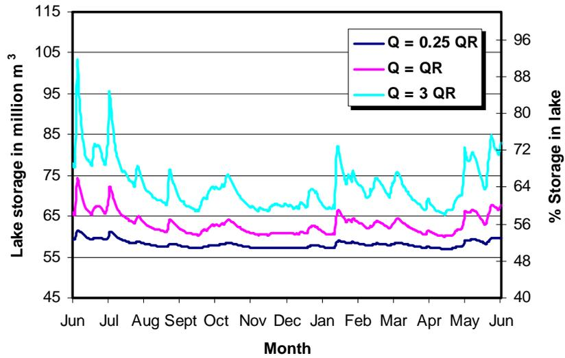
Figure 16. Black Lake water storage for the present exit base-level ( $E_{le} = 998.75\text{m}$ ;  $S = 55$  millions  $\text{m}^3$ ) under different flow events,  $Q_R = 18.9 \text{ m}^3/\text{s}$ .
