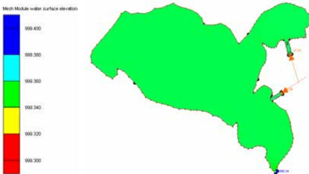
Figure 20. Water surface elevation in the lake (event-1);  $Q_T = 68.16 \text{ m}^3/\text{s}$ ; dimensions in m.
