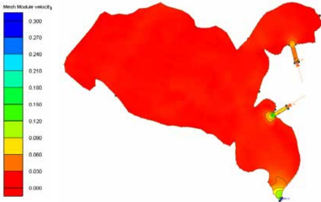
Figure 23. Velocity distribution in the lake and its inlets and exit (event - 2);  $Q_T = 20.42$   $\text{m}^3/\text{s}$ ; dimensions in m/s.
