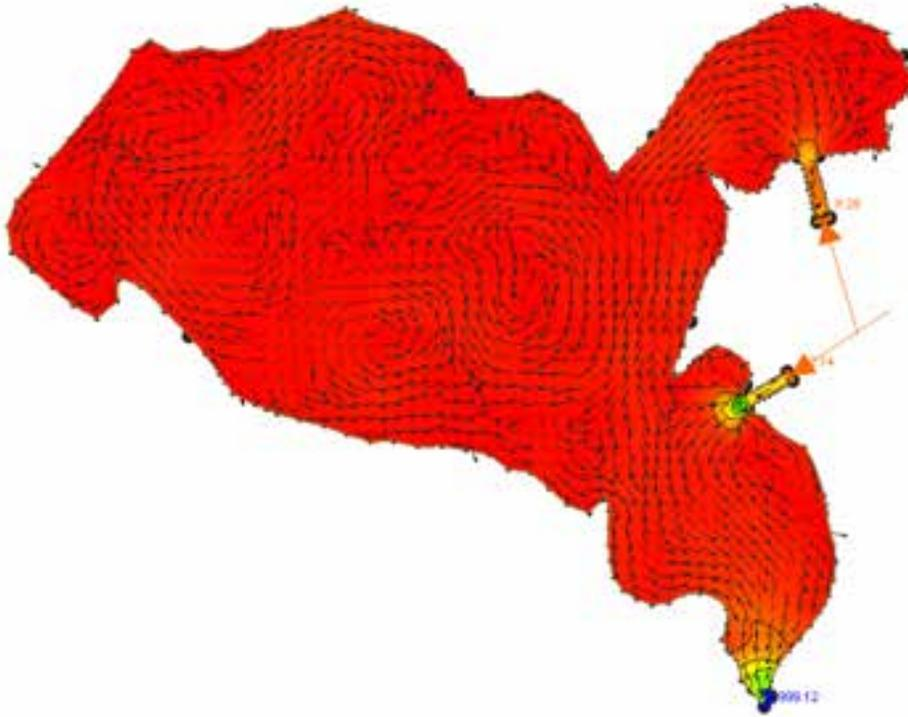
Figure 29. Re-circulation pattern for event -2;  $Q_T = 20.42 \text{ m}^3/\text{s}$ .
