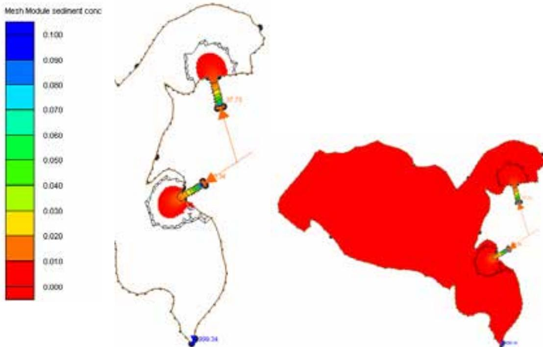
Figure 26. Sediment concentration distribution in the lake and its inlets and exit (event – 1);  $Q_T = 68.16 \text{ m}^3/\text{s}$ ; dimensions in  $\text{ppm} \times 10^3$ .
