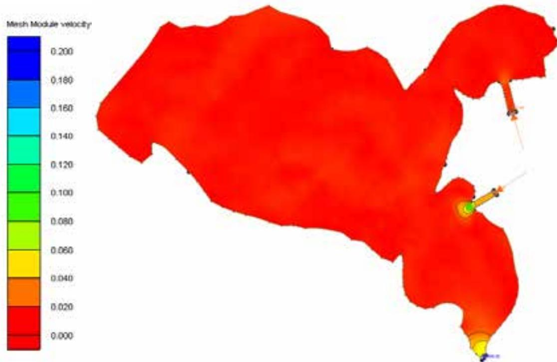
Figure 24. Velocity distribution in the lake and its inlets and exit (event - 3);  $Q_T = 8.74$   $\text{m}^3/\text{s}$ ; dimensions in m/s.
