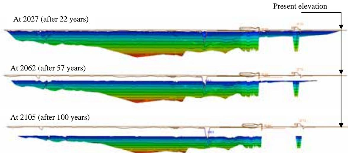
Figure 35. Expected possible changes in the Black Lake water surface elevation over a period of 100 years.
