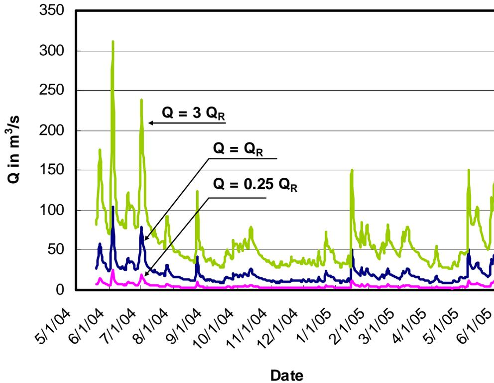
Figure 9. Range of the generated time series with respect to the reference discharge,  $Q_R = 18.9 \text{ m}^3/\text{s}$ .
