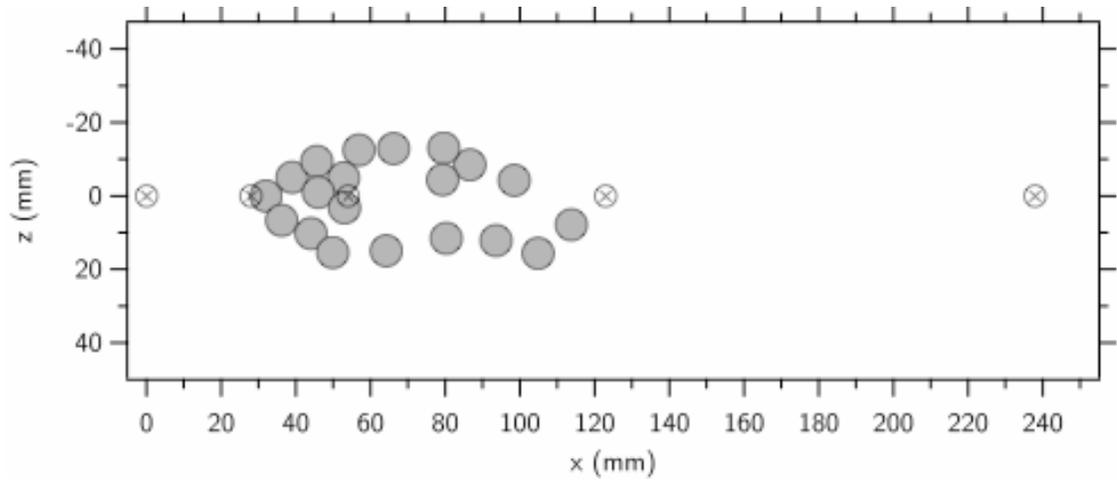
**Figure 3:** Plan view of the single cluster domain. Flow is from left to right, and points marked by  $\otimes$  represent the velocity profile locations.  $x=0$  mm = region 1,  $x=28$  mm = region 2,  $x=54$  mm = region 3,  $x=123$  mm = region 4, and  $x=238$  mm = region 5.
