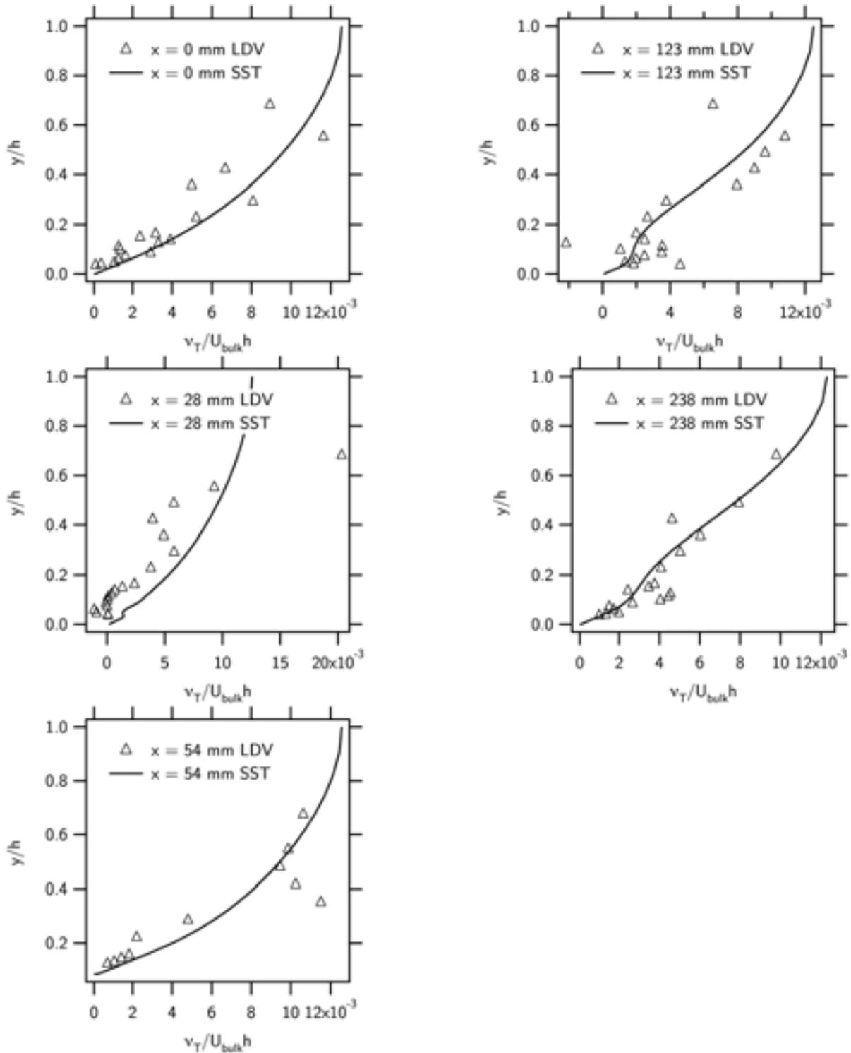
**Figure 13:** Comparison of experimental and numerical simulation for  $v_T$  at: (a)  $x=0$  mm, (b)  $x=28$  mm, (c)  $x=54$  mm, (d)  $x=123$  mm, and (e)  $x=238$  mm.
