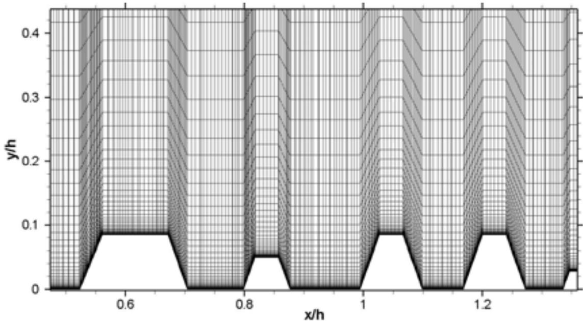
**Figure 9:** Mesh spacing in the vertical and horizontal along the plane  $z=0.162h$  ( $z=12.5$  mm).
