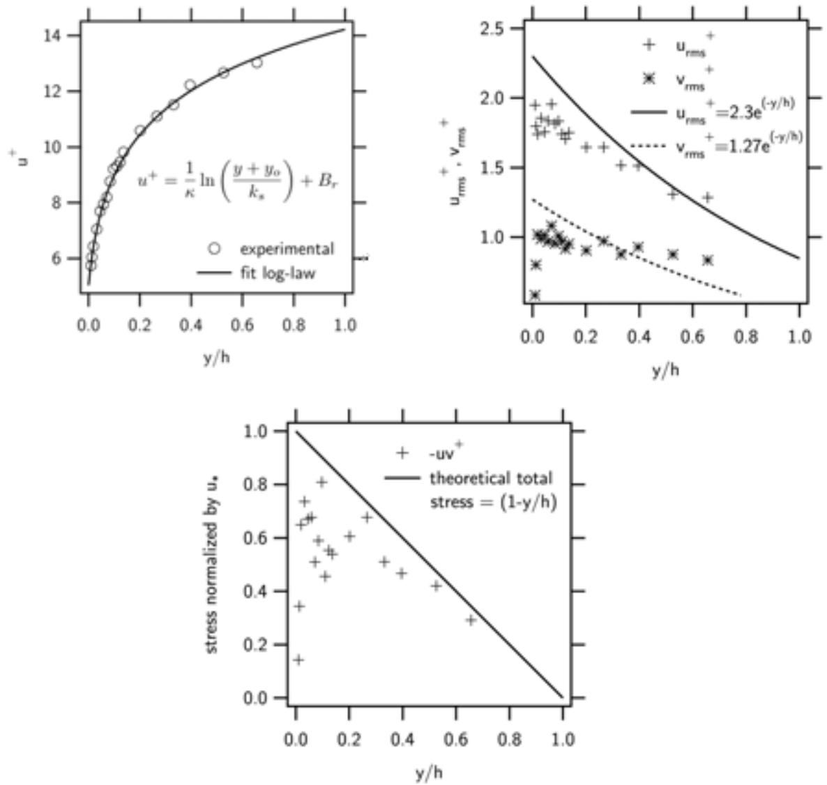
**Figure 5:** Experimental data. (a) streamwise velocity at  $x=0$  mm compared with Eq. 5; (b) turbulent intensities at  $x=0$  mm compared to Eq. 4.3 and 4.4 of Nezu and Nakagawa; and (c) Experimentally measured Reynolds stress  $-uv^+$  at  $x=0$  mm compared to the 2D uniform open channel theoretical total stress (turbulent + viscous stress) distribution.
