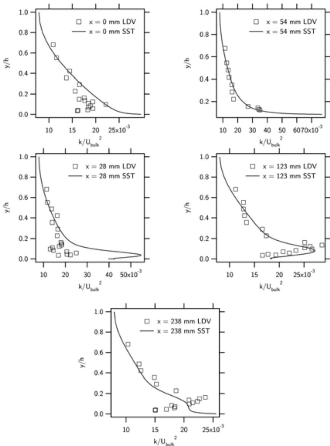
**Figure 12:** Comparison of experimental and numerical simulation for  $k$  at: (a)  $x=0$  mm, (b)  $x=28$  mm, (c)  $x=54$  mm, (d)  $x=123$  mm, and (e)  $x=238$  mm.
