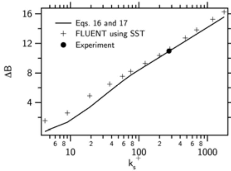
**Figure 6:** SST near-wall model predicted response of  $\Delta B$  to changes in roughness,  $k_s^+$ , compared to Eqs. 16 and 17.
