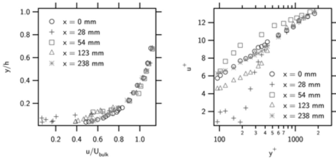
**Figure 4:** Experimentally measured velocity profiles at  $x=0$  mm: approach velocity,  $x=23$  mm: decelerated stoss region,  $x=54$  mm: atop cluster,  $x=123$  mm: wake,  $x=238$  mm: return to unaffected state.
