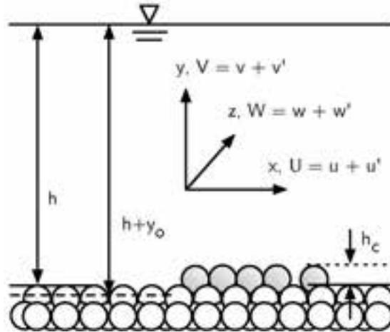
**Figure 1:** Coordinate system definition; vertical slice schematic. Grey particles represent a formed cluster atop the uniform roughness bed.
