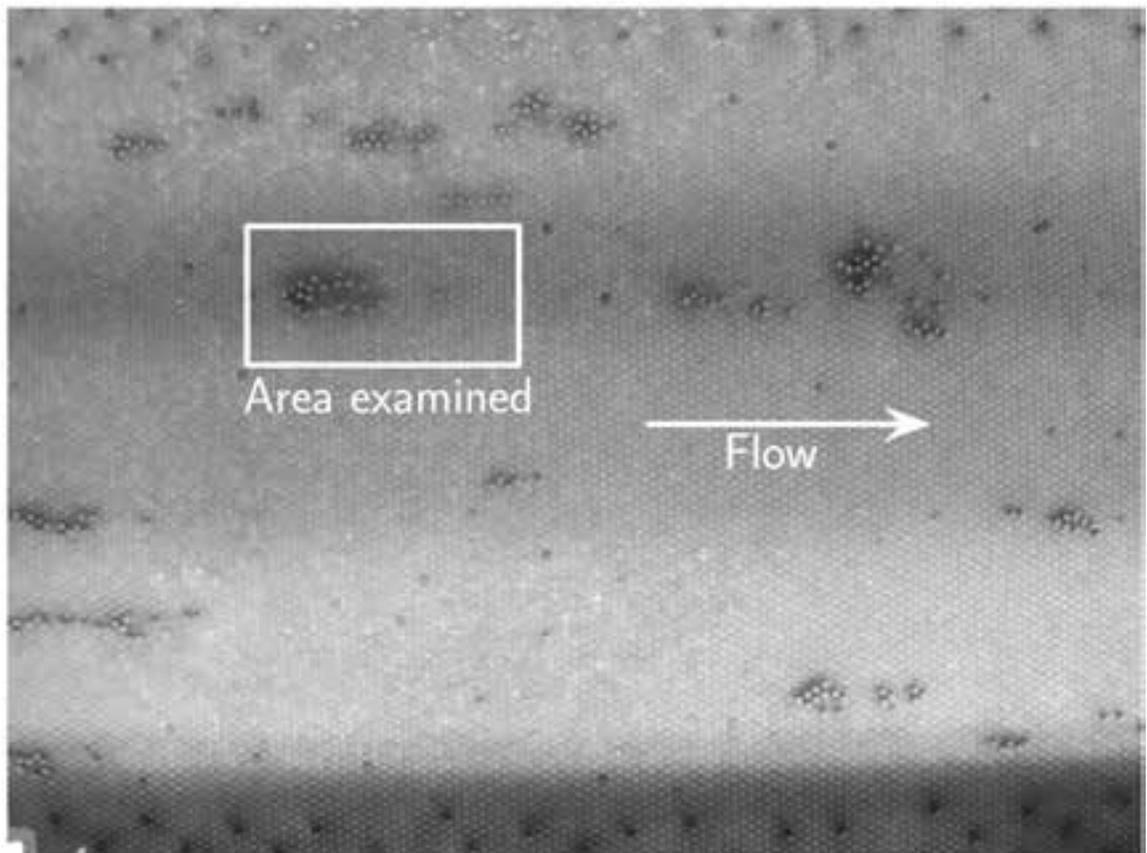
**Figure 2:** Plan view of self-occurring clusters. Light colored particles are the uniform roughness bed and the darker particles are the formed clusters and individual sediment particles.
