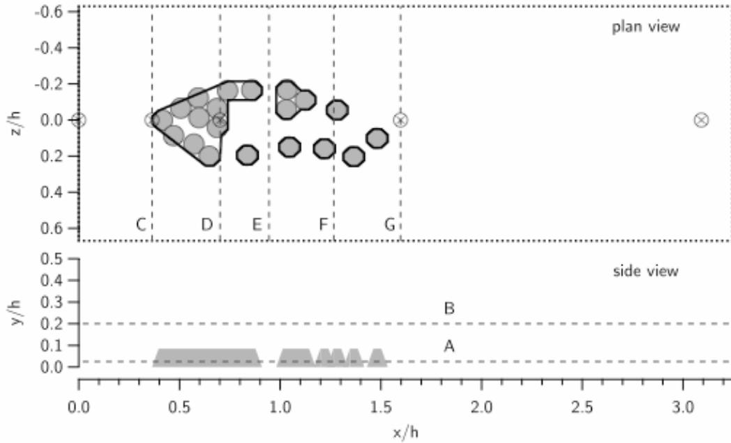
**Figure 8:** Footprint and side view of cluster mesh compared to the experimental cluster along with the location of key planes (A-G) examined in the solution. Grey spheres represent the experimentally formed cluster, the black overlaid line represents the footprint of the computational mesh, dotted lines are planes examined in the solution, and  $\otimes$  marks the experimental velocity profile locations.
