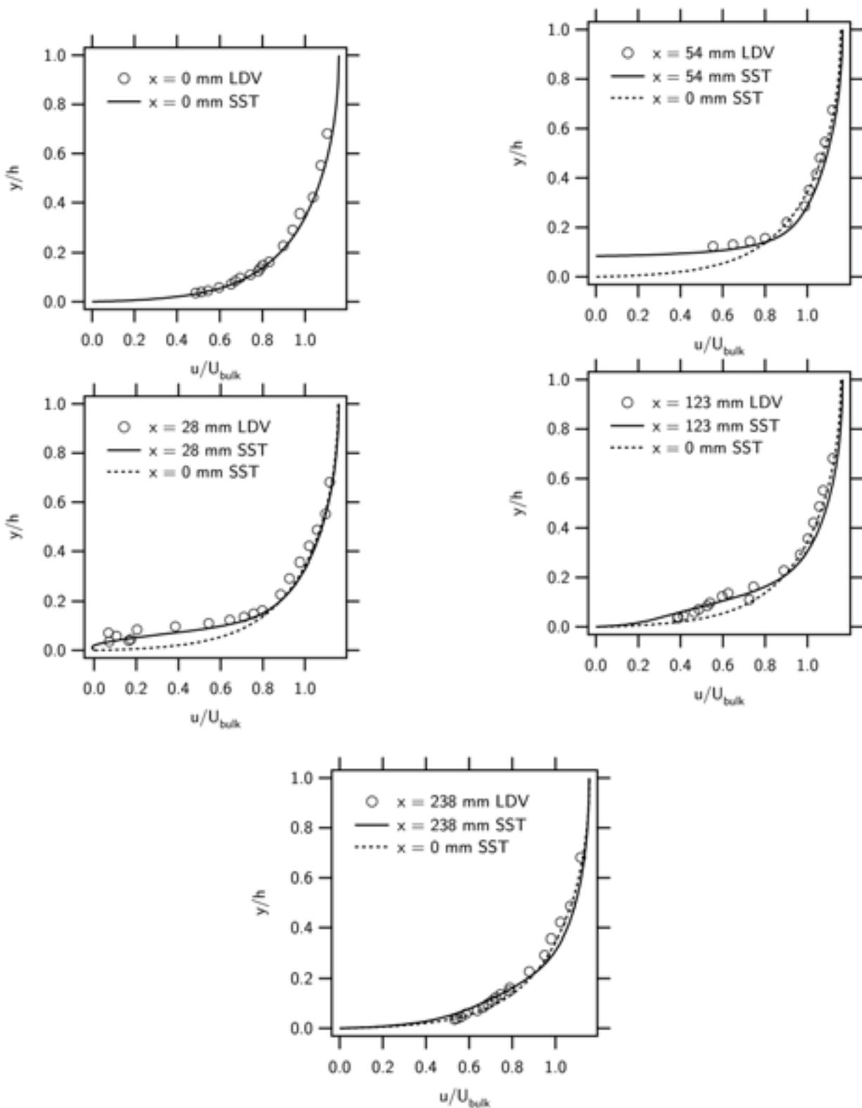
**Figure 11:** Comparison of experimental and numerical simulation for  $u$  at: (a)  $x=0$  mm, (b)  $x=28$  mm, (c)  $x=54$  mm, (d)  $x=123$  mm, and (e)  $x=238$  mm.
