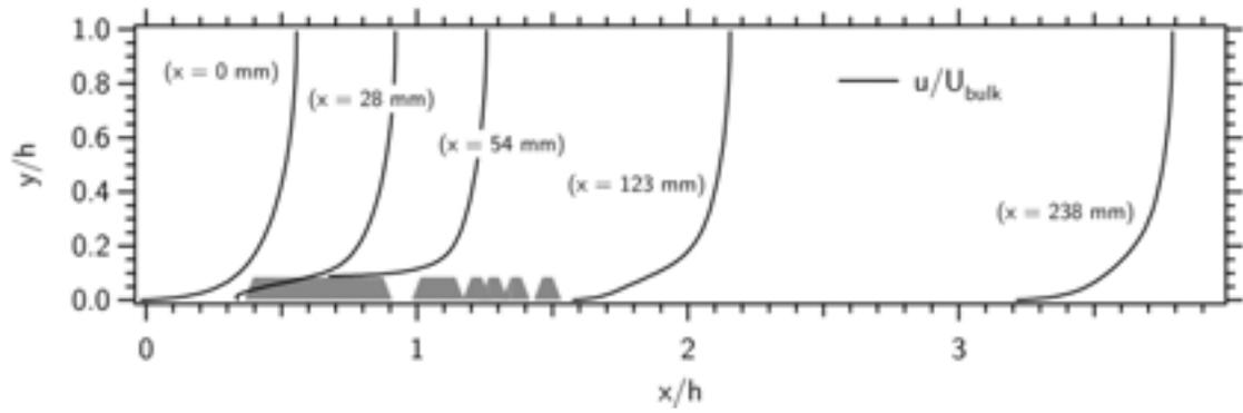
**Figure 10:** Velocity profiles over cluster as predicted by the SST near-wall solution.
