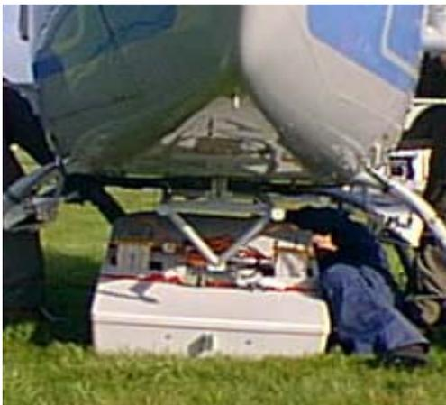
Figure 9: Installation of a GPR under a helicopter during the Cowlitz River experiment in May 2001
