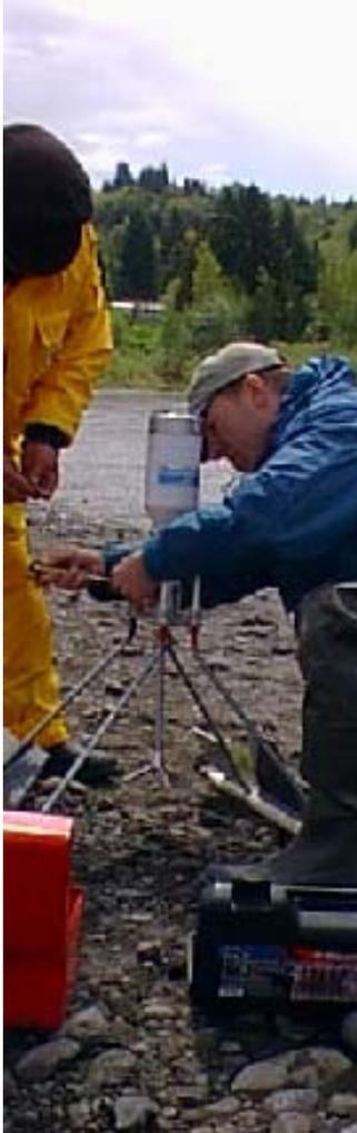
Figure 12: SonTek ADCP probe with converging beams on the bank of the Cowlitz River on the 1<sup>st</sup> of May 2001.
