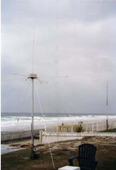
Figure 3: Bi-static radar SeaSonde® by Codar in operation on a beach.
