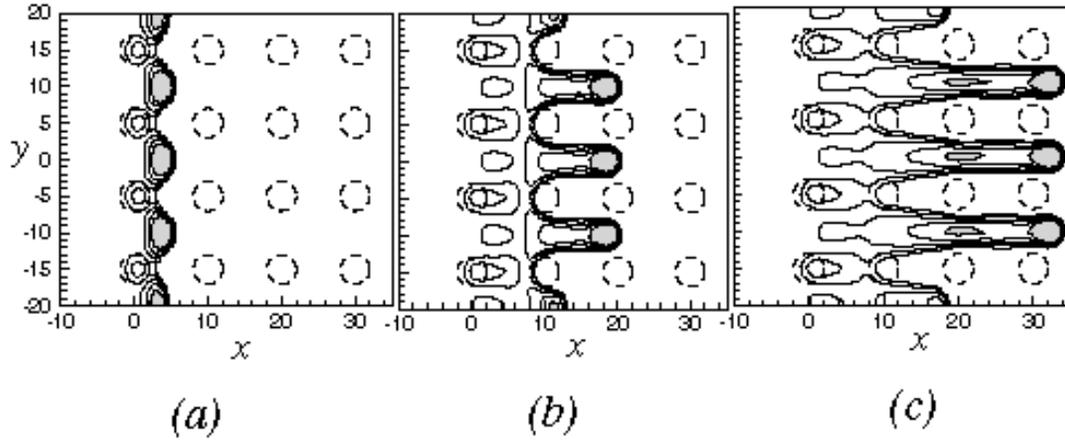
Figure 25. Contour plots of the layer thickness showing rivulet development for passage of a driven front through a symmetric array of positive relative contact angle spots, at times (a)  $t = 5$ , (b)  $t = 15$ , and (c)  $t = 24$ .
