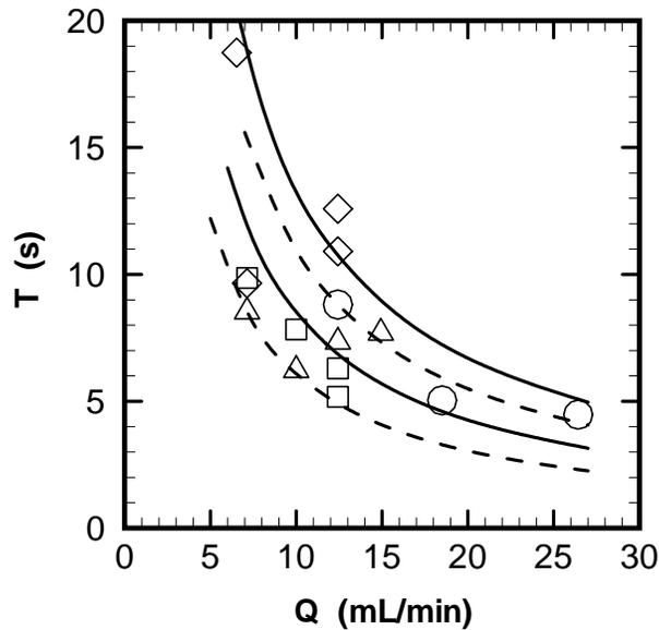
Figure 12. Period of rivulet break-off for partial-gravity cases as a function of water flowrate with air speed held constant at 11 m/s, for cases with 0 g (squares), 0.16 g (deltas), 0.26 g (circles), and 0.38 g (diamonds). Curves are predictions from Eqn. (1) with  $C = 0.05$  (lower dashed), 0.07 (lower solid), 0.09 (upper dashed), and 0.11 (upper solid), respectively.
