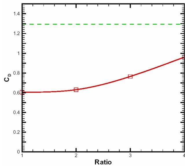
Figure 16. Variation of drag coefficient of a hemi-ellipsoid with aspect ratio for  $Re = 6000$ . Limiting two-dimensional case is indicated by a dashed line.
