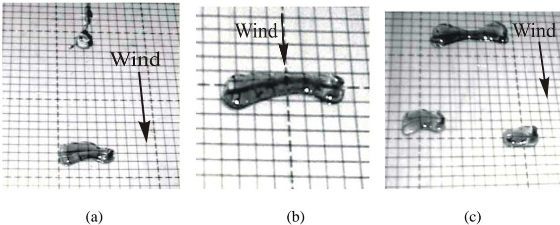
Figure 5. Examples of downstream-propagating droplets on a horizontal surface in 1g: (a) droplet shortly after break-off from rivulet, (b) close-up view of the elongated, double-lobe structure of the droplet, and (c) a larger droplet overtaking two smaller droplets. Wind flow is from top to bottom.
