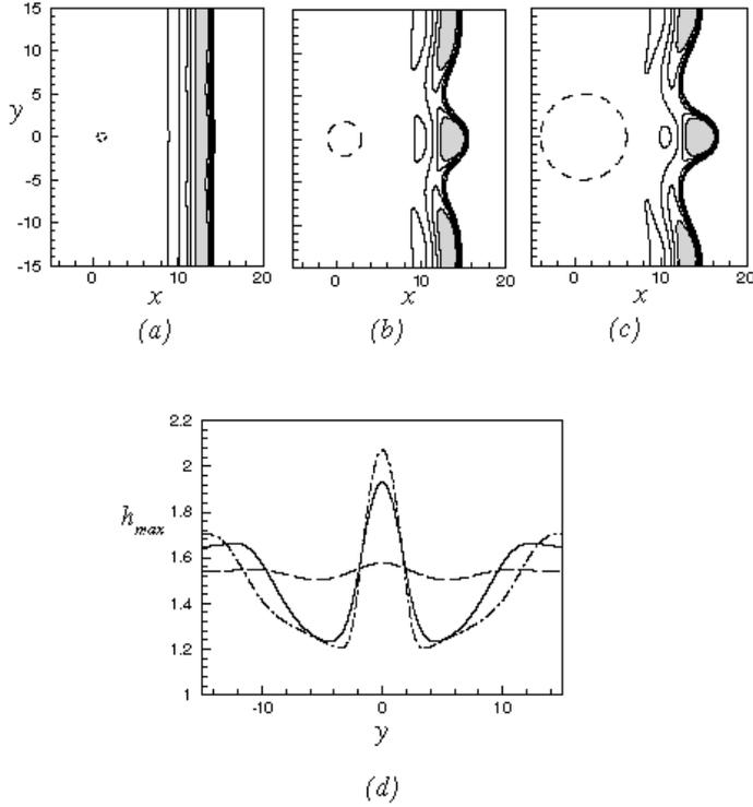
Figure 24. Contours of layer thickness showing effect of contamination spot radius on the liquid layer at time  $t = 15$  for cases with (a)  $R = 0.5$ , (b) 2.0, and (c) 5.0. The profile of the maximum value of layer thickness is plotted versus  $y$  at the same time in Figure (d) for  $R = 0.5$  (dashed curve), 2.0 (solid curve) and 5.0 (dashed-dotted curve).
