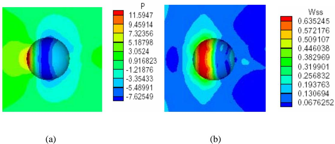
Figure 14. Distribution of (a) pressure and (b) shear stress on a hemisphere attached to a flat surface with  $Re = 6000$ . Flow is from left to right.
