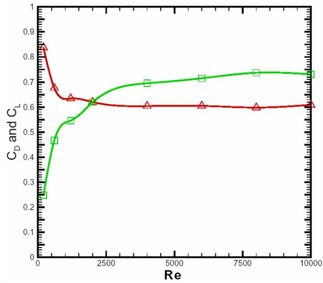
Figure 15. Variation of drag coefficient (triangles) and lift coefficient (squares) with Reynolds number for a hemisphere attached to a flat surface.
