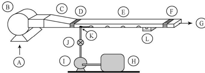
Figure 1. Sketch of the rivulet wind tunnel showing (A) air inlet, (B) blower, (C) contraction, (D) honeycomb, (E) test section, (F) honeycomb water trap, (G) air outlet, (H) collapsible water storage tank, (I) positive-displacement pump, (J) needle valve, (K) water inlet hole, (L) water collection box.
