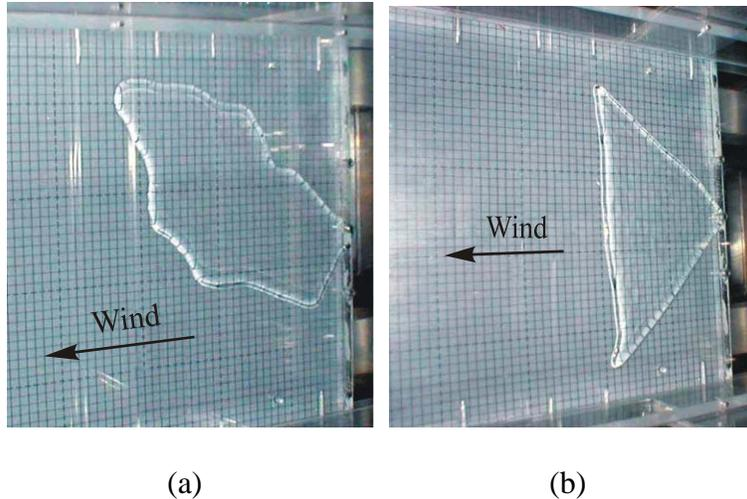
Figure 2. (a) At very low wind speeds, a puddle of water forms around the water outlet and spreads downwind; (b) increasing wind speed causes the puddle to become fan-shaped. The surface is horizontal in both cases.
