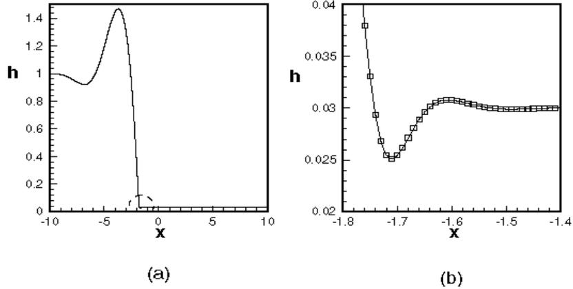
Figure 17. Plots of (a) equilibrium layer thickness profile versus position along the substrate and (b) a close-up showing the overshoot in layer thickness in the region indicated by a dashed half-circle in (a). The symbols in (b) are the numerical computation points.
