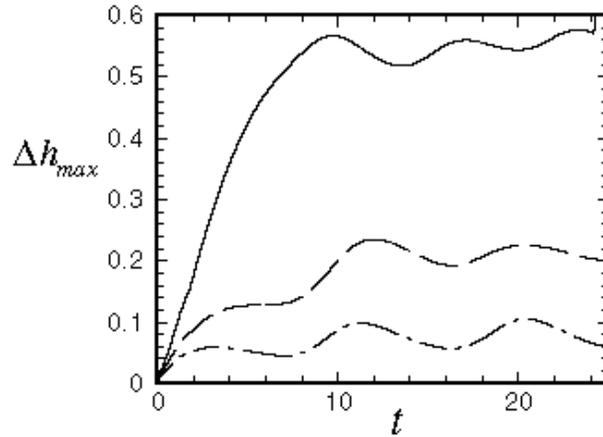
Figure 30. Effect of  $P_2$  on time variation of the change in maximum layer thickness for cases with  $P_2 = 0$  (solid curve),  $P_2 = 1$  (dashed curve), and  $P_2 = 2$  (dashed-dotted curve).
