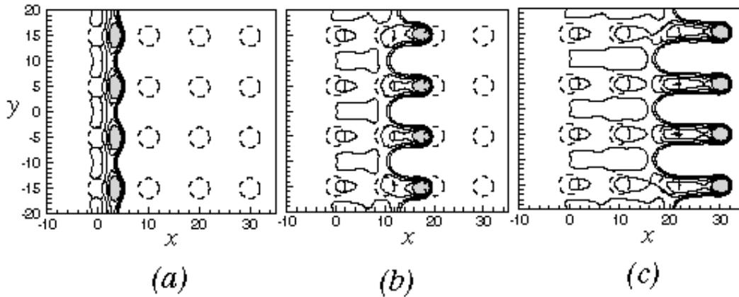
Figure 26. Contour plots of the layer thickness showing rivulet development for passage of a driven front through a symmetric array of negative relative contact angle spots, at times (a)  $t = 5$ , (b)  $t = 15$ , and (c)  $t = 24$ .
