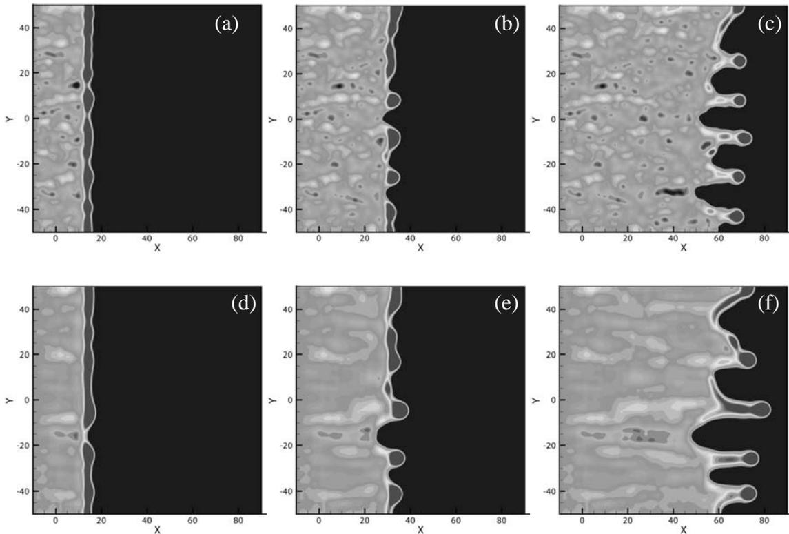
Figure 32. Results for finger growth on a driven liquid film over a surface with contact angle variation with correlation length  $\ell = 4$  (a-c) at times  $t = 15, 30,$  and  $60,$  and with correlation length  $\ell = 16$  (d-f) at the same three times.
