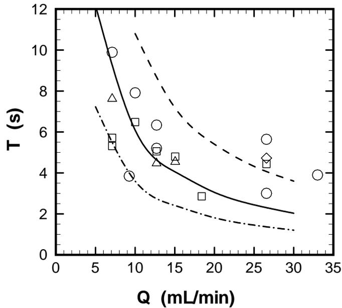
Figure 8. Period of rivulet break-off in zero-gravity versus the water discharge rate, for cases with  $Q = 10.3$  mL/min (squares),  $11.4$  mL/min (deltas),  $11.9$  mL/min (circles), and  $12.5$  mL/min (diamonds). The curves give the theoretical predictions from Eqn. (1) with  $C = 0.05$  for  $U = 10$  m/s (dashed),  $11$  m/s (solid) and  $12$  m/s (dashed-dotted).
