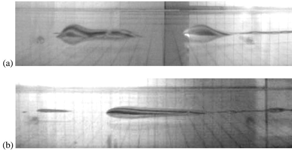
Figure 11. Photographs of the rivulet head and detached droplets for (a) 0.38g ( $Q = 10$  mL/min,  $U = 11$  m/s) and (b) 1.5g ( $Q = 10$  mL/min,  $U = 12.4$  m/s).
