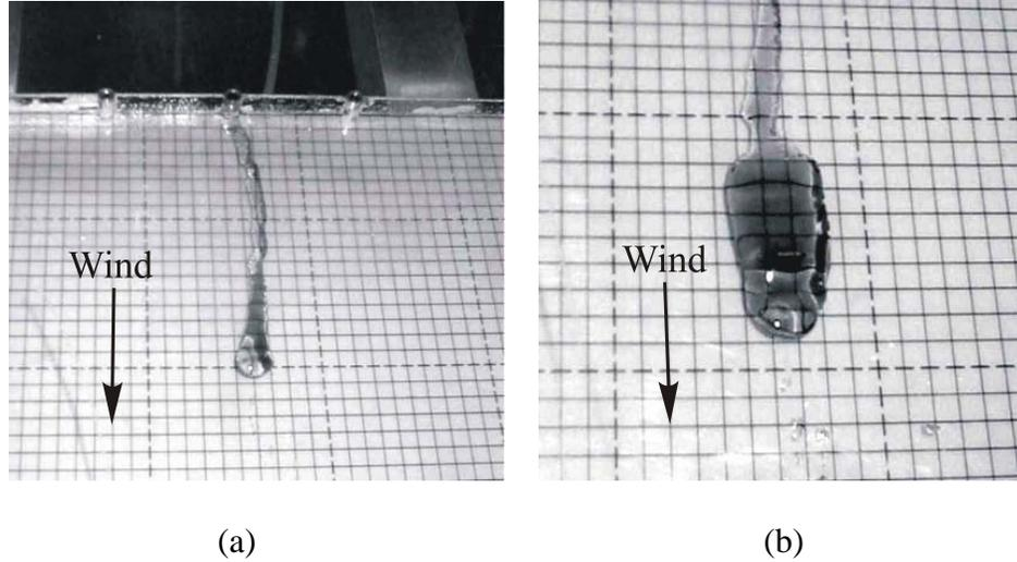
Figure 3. Photographs showing break-up of a wind-driven rivulet to form a droplet in 1g, including (a) the rivulet at a time where it has stopped progressing and is beginning to form a large droplet, and (b) close-up of the droplet about to detach from the rivulet. Wind flow is from top to bottom.
