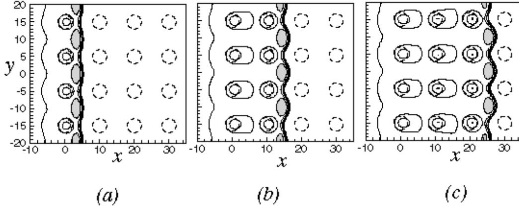
Figure 29. Time series showing contour lines of layer thickness for a case with  $P_2 = 2$  and a symmetric array of positive relative contact angle spots, at times (a)  $t = 5$ , (b)  $t = 15$ , and (c)  $t = 25$ . Five evenly spaced contours are plotted over the interval  $(0.7, 1.1)$ , and gray shading indicates regions where  $h > 1.1$ .
