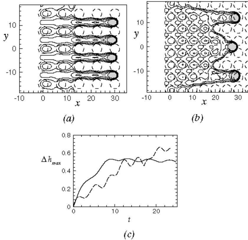
Figure 27. Plots illustrating passage of a driven layer front through a symmetric array of positive relative contact angle spots with spacing  $\lambda$  less than the critical value for instability: (a) case with  $\lambda = 7.5$  showing sub-critical instability induced by contamination spots, (b) case with  $\lambda = 5$  showing rivulet develop with spacing greater than  $\lambda$ , (c) time variation of change in maximum layer thickness for (a) (solid curve) and (b) (dashed curve).
