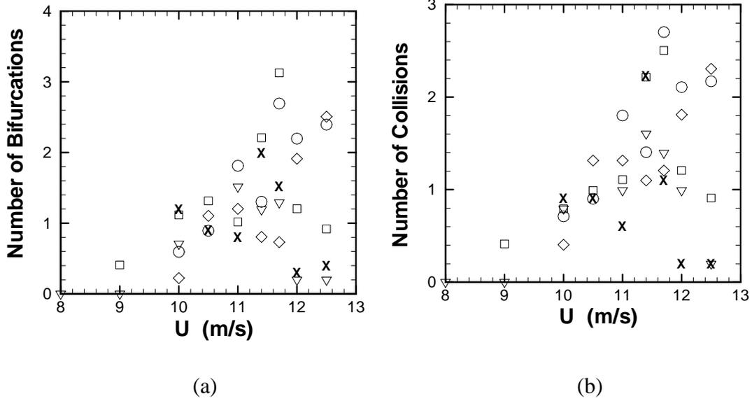
Figure 6. Graphs of droplet bifurcations and collisions for the terrestrial gravity experiments, showing average number of times a single droplet (a) bifurcates and (b) collides with another droplet as it traverses the test surface for cases with water flow rate  $Q = 5$  mL/min (crosses), 10 mL/min (squares), 15 mL/min (deltas), 20 mL/min (circles), and 40 mL/min (diamonds).
