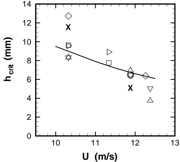
Figure 9. The average height of the rivulet head at the break-off time for all zero-gravity experiments, where  $Q = 7$  mL/min (squares), 10 mL/min (deltas), 12.5 mL/min (gradients), 18.5 mL/min (right triangles), 26.5 mL/min (crosses), 33 mL/min (circles). The curve represents the theoretical prediction from Eq. (2) with  $A = 3.7$ .
