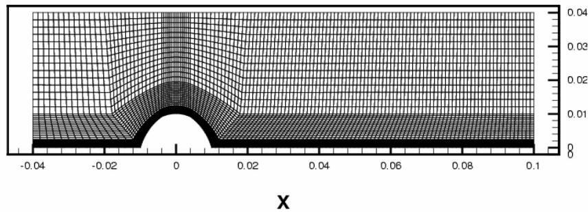
Figure 13. Section view of three-layer uniform grid at  $y = 0$  used for simulation of air flow over a hemisphere.
