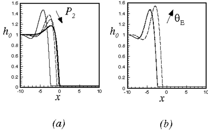
Figure 18. Variation of equilibrium layer profiles with (a) normal body force and (b) contact angle. Figure (a) shows cases with  $P_2 = 0$  (upper solid curve), 0.5 (dashed curve), 1.0 (dashed-dotted curve) and 2.0 (lower heavy solid curve). Figure (b) shows cases with  $\theta_E = 0$  (lower solid curve), 0.1 (dashed-dotted curve, coincident with the  $\theta_E = 0$  case), and 0.3 (dashed-dotted curve).
