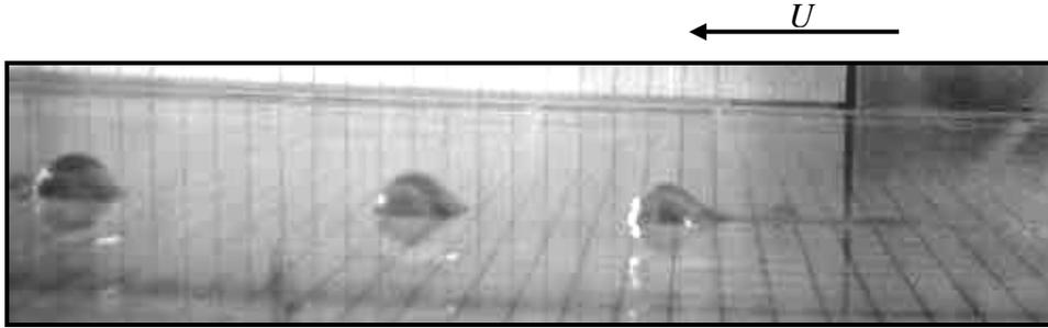
Figure 7. Periodic shedding showing two nearly hemispherical droplets with a third about to break off from the end of the rivulet for zero-gravity case ( $Q = 15$  mL/min,  $U = 11.8$  m/s). The grid lines have a spacing of 6 mm.
