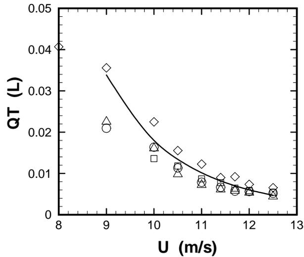
Figure 4. Data for (a) rivulet break-off period  $T$  and (b) product of rivulet break-off period  $T$  and the water flow rate  $Q$  versus air speed  $U$  for the terrestrial gravity (1g) case, for values of water flow rate of  $Q = 10$  mL/min (squares), 15 mL/min (deltas), 20 mL/min (circles), and 40 mL/min (diamonds). The solid line is the theoretical prediction given by Eqn. (1) with  $C = 0.5$ .
