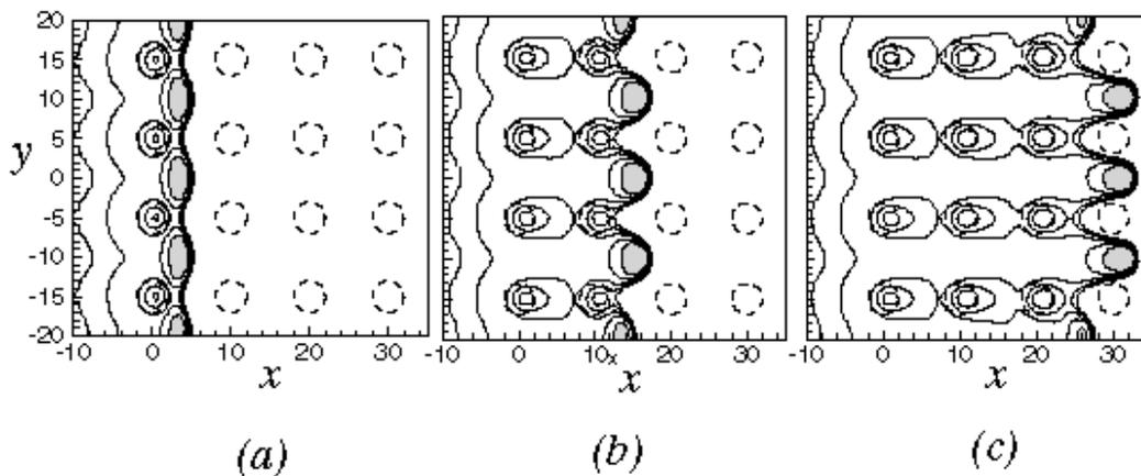
Figure. 28. Time series showing contour lines of layer thickness for a case with  $P_2 = 1$  and a symmetric array of positive relative contact angle spots, at times (a)  $t = 5$ , (b)  $t = 15$ , and (c)  $t = 25$ . Five evenly spaced contours are plotted over the interval  $(0.8, 1.2)$ , and gray shading indicates regions where  $h > 1.2$ .
