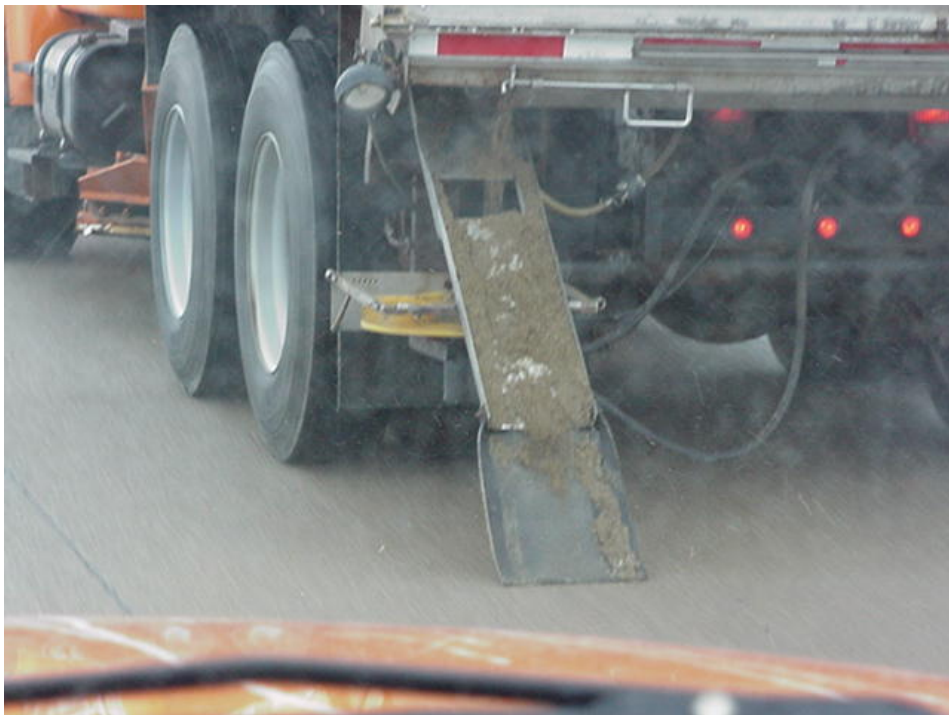
Figure 2.28. Sander chute in by-pass mode
