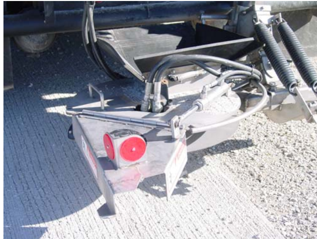
Figure 2.5. Truck D - standard truck from the Oakdale shop that was equipped with a Swenson Positive Placement System (PPS) zero velocity unit.
