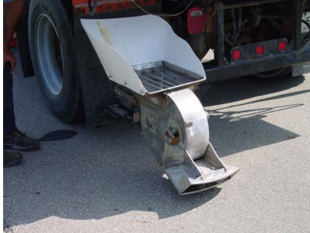
Figure 2.4. Truck C - Monroe Accuspread zero velocity system. The truck is a standard truck from the fleet equipped with a prototype Accuspread unit modified by the Bedford shop.
