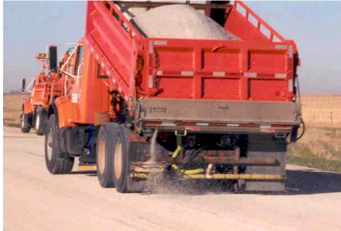
Figure 2.2. Truck A - standard truck with traditional tailgate spreader that would be typical of the department's fleet. Spreader was mounted on the left hand side of the truck, approximately 18 inches from the roadway surface.
