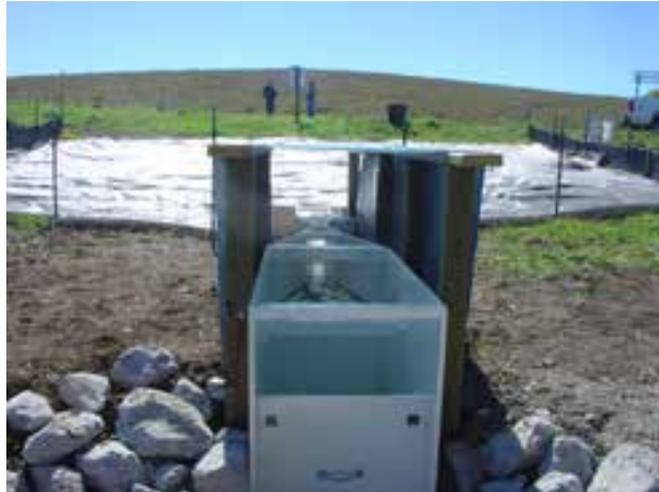
Figure 9d – Parshall flume
