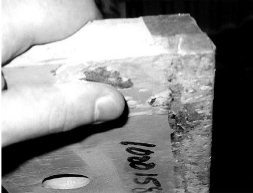
Figure 1b. SHRP cutting edge, with exposed carbide insert in leading edge.
