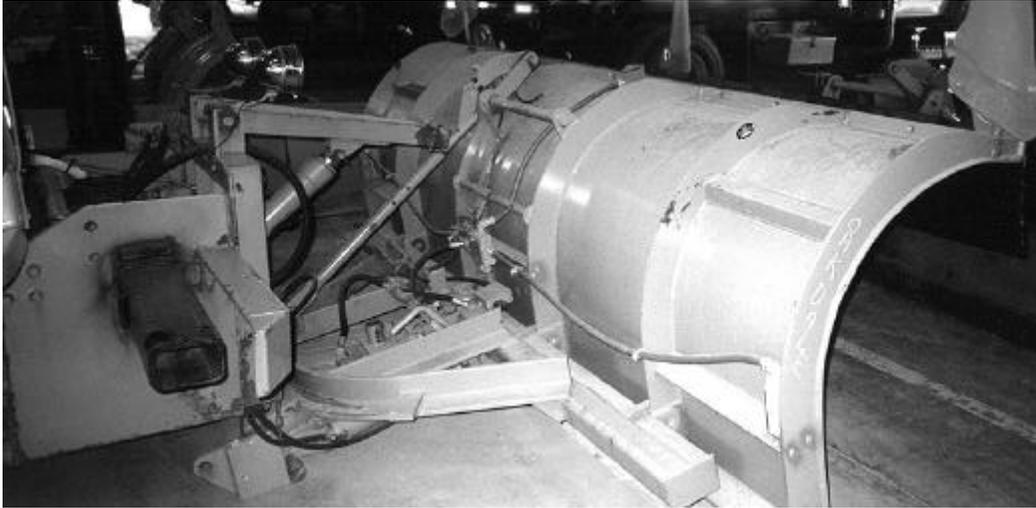
Figure 7a. The front plow, with accelerometers mounted in the metal boxes.
