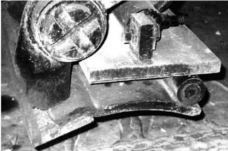
Figure 5. The actual underbody plow, showing both cutting edge and the inclinometer.
