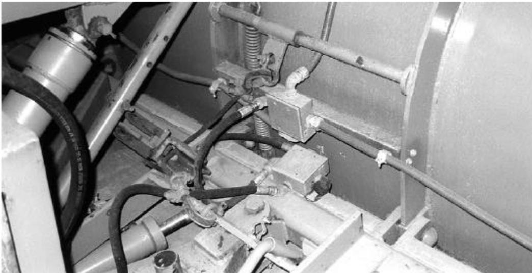
Figure 7b. Detail of the protective mounts for the accelerometers.
