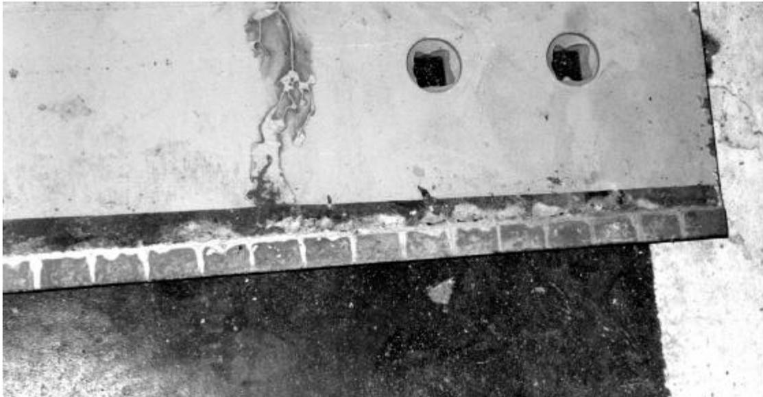
Figure 2. Segmented nature of the carbide insert in the SHRP cutting edge.
